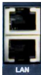
LAN (lower) and ETHERNET (top) connectors
